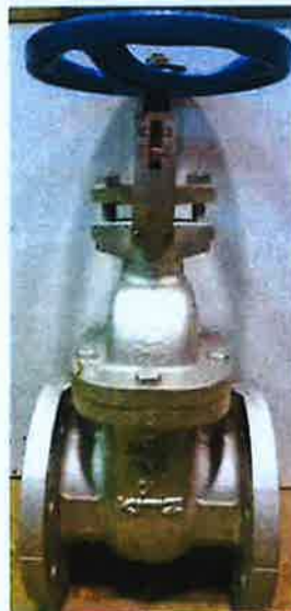
Photo 1. "KITZ" brand cast iron gate valve, non-rising stem, metal seated, with position indicator, flanged PN16 (Category 1) silver color coated outside.
